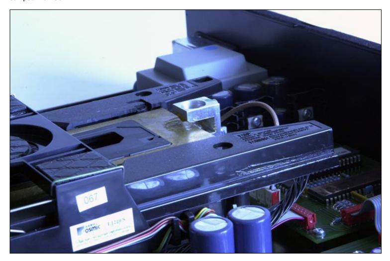
Gyropoint technology thus becomes a means to secure the CD better in the transport as well as to offload any mechanical vibration to the CD player's frame. But that's not all. All mechanical parts of the player are covered with heavy, inert bitumen, again to get rid of spurious vibrations.
